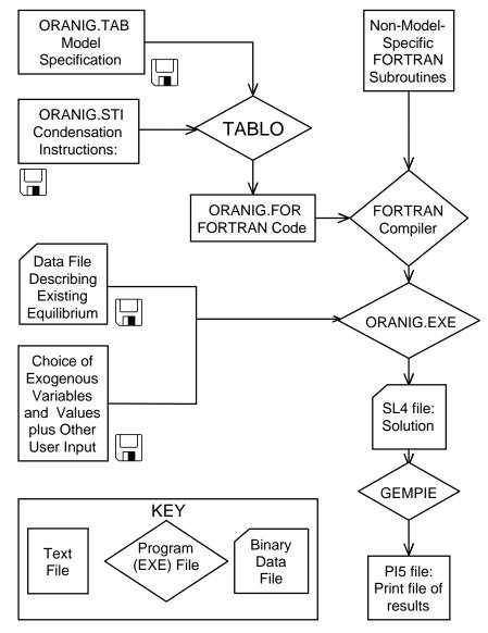
Figure 8. Stages in the GEMPACK process
